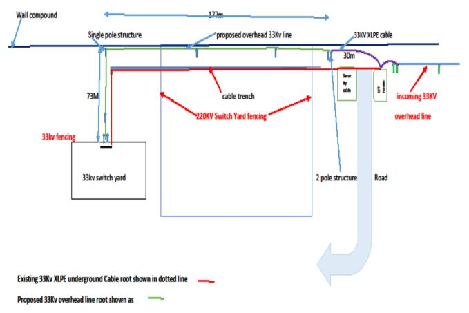
(Total conductor length for proposed 33KV overhead = 73+177= 250 Meter.)
